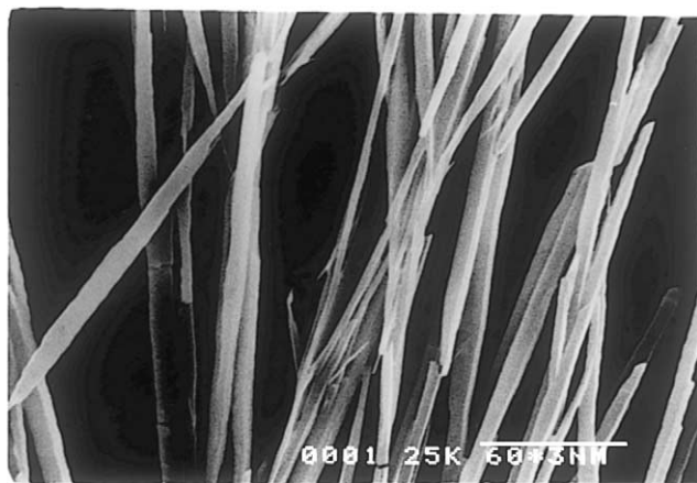
Figure 4. SEM image of the peptide 1 showing filamentous fibrillar morphology in the solid state.
